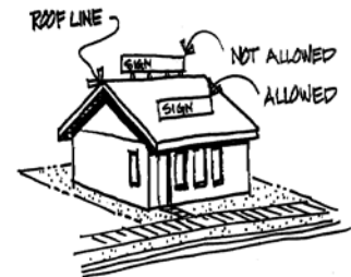
Roof Line and Roof Sign
