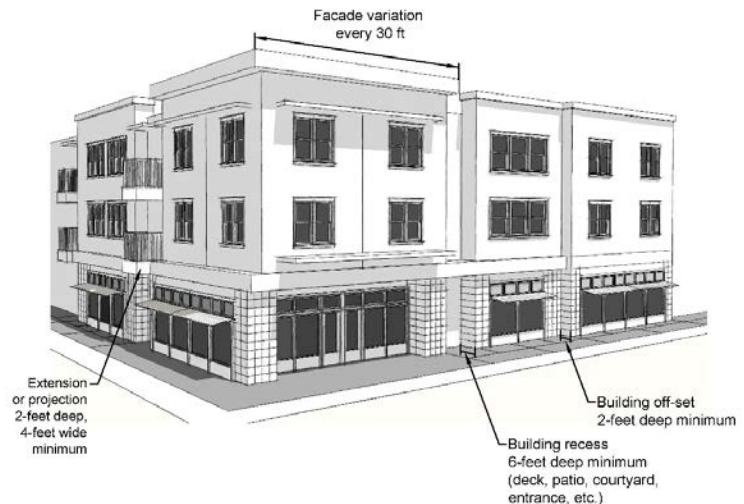
Figure 2.130.10.I-1: Façade Variation and Detailing
