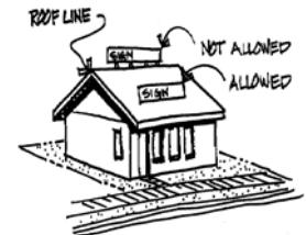
Roof Line and Roof Sign
